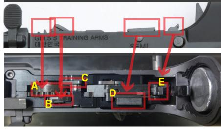
A: 3RD GEAR SET | B: GEAR STOPER | D: AUTO CONTROLLER | E: SEAR
